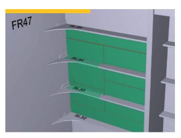
The SPS was applied from the inside with a 12mm top plate welded to the framing members. Most hot work took place away from the side shell. The SPS elastomer core was injected into the resulting cavity to form the composite sandwich.
