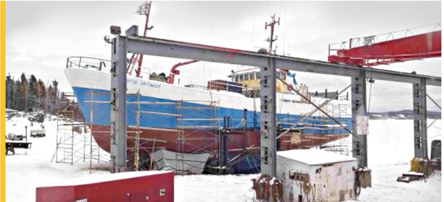
➔ The existing steelwork on board the vessel was badly corroded, access tight and a crop-and-replace repair was an unattractive option.
